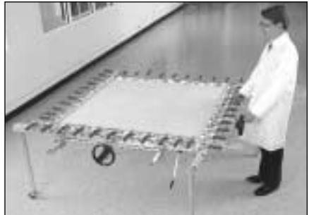
*The H24-D is a highly precise, self-contained, continuously adjustable tensioning system. It is especially suited to thick film and surface mount screens and masks, glass and containers, precision graphics and electronics.*
