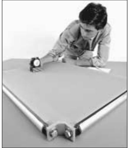
*The use of a tension meter is critical in assuring uniform and optimum screen tension levels.*
