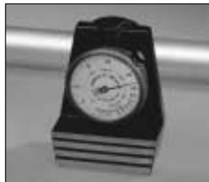
*Monitor screen tension easily and accurately with the Newman ST-Meter®.*
