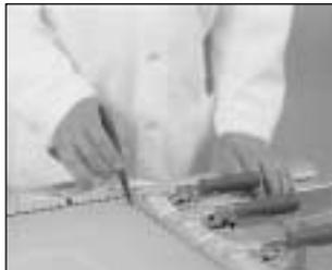
Use clamp edge as a guide for marking adjustment line.
