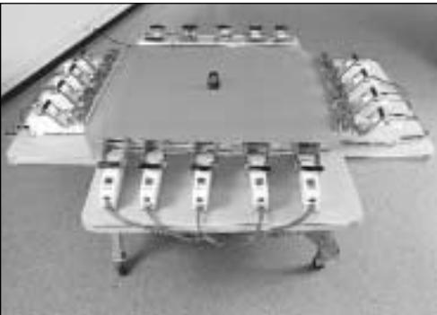
Saati pneumatic clamps employ a unique "movable" design for "contact-less" uniform tensioning.
