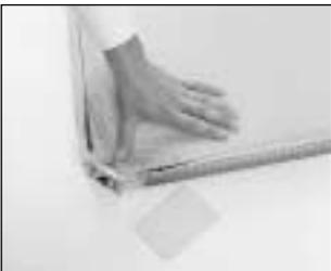
Check for uniformity measuring angle adjustment from both rollers.
